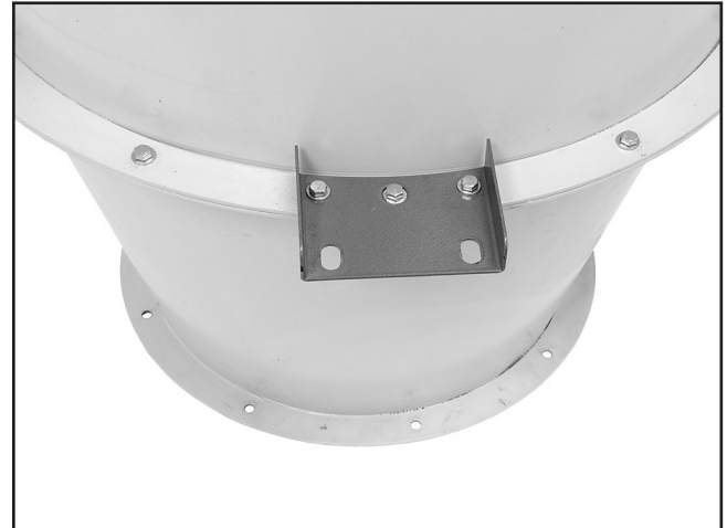
Figure 19. Cyclone mounting bracket mounted to collector assembly.
